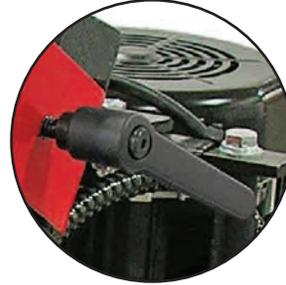
**SAVE TIME:** ADJUSTABLE RETRACTION STOP LIMITS RAM RETRACTION.
