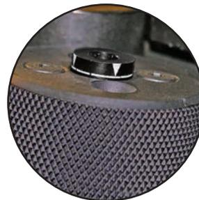
**ACCURATE AND REPEATABLE:** AN INFINITELY ADJUSTABLE MICROMETER AND THE MICRO SITE INDICATOR MAKE PRECISE AND REPEATABLE CRIMPS.
