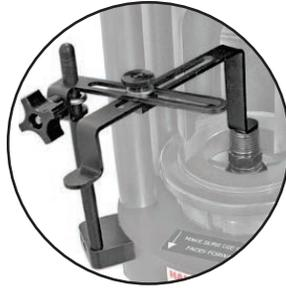
**SAVE TIME:** REMOVABLE FITTING STOP FOR MULTIPLE CRIMPS OF THE SAME HOSE AND FITTING.
